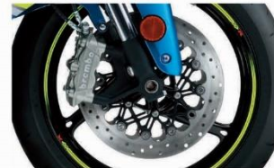
Radial-mount Brembo monoblock calipers
